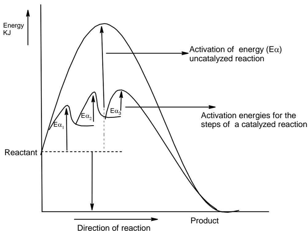
**Fig. 6: Figure comparing the quantum of energy of activation in case of uncatalyzed and various steps of catalyzed reaction.**
