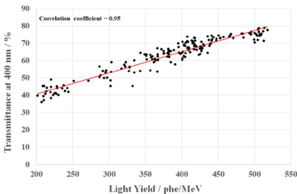
**Fig. 2.** Correlation between the optical transmission at 400 nm of the samples of 0.5 cm thick and the light yield measured at room temperature using a PMT with bialkali photocathode. Samples have been produced at the pre-production run with concentration of Ce<sub>2</sub>O<sub>3</sub> 0.76 weight %.
