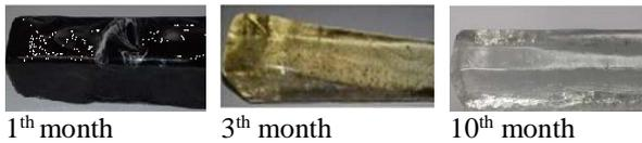
**Fig.1.** Ce-doped DSB-Gd bulks after technology development for 1, 3 and 10 months.
