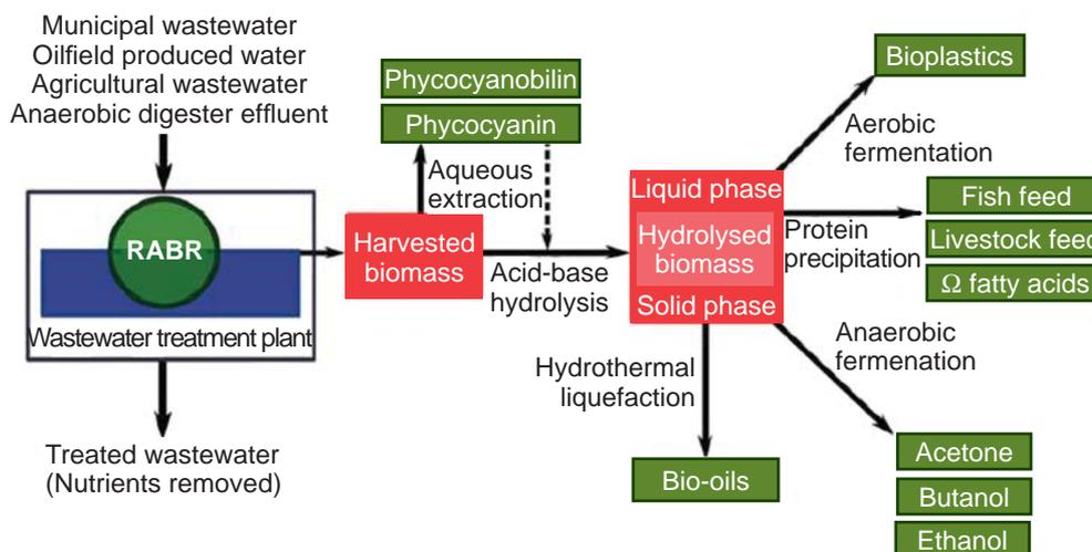
Fig. 1. Coupling wastewater treatment with algae production (Reproduced by permission of Springer India)
